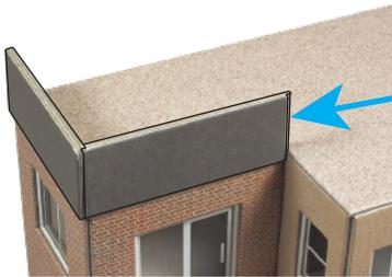
Now add RW2 this slots into the end of RW1, and flush to the roof edge.
