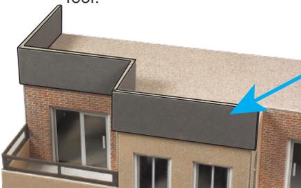
Now add the centre section, RW4, flush to the roof edge and overlapping the end of RW3.
