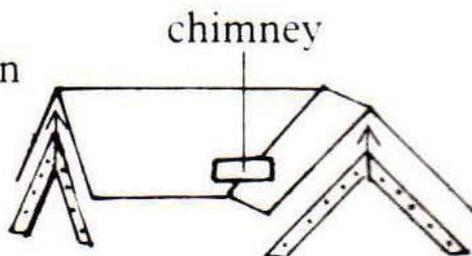
Glue chimney halves together and trim tops to square the pots. Each chimney should line up with, and glue to the supporting wall.
