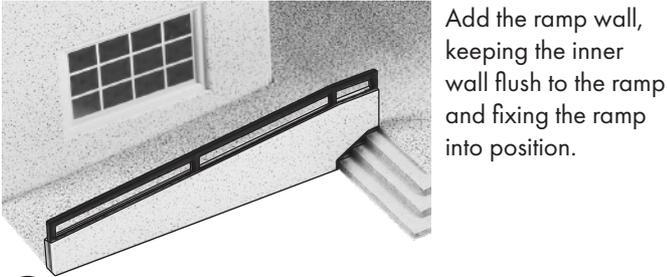
Add the ramp wall, keeping the inner wall flush to the ramp and fixing the ramp into position.
